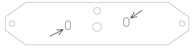
To fit a badly made OEM pickup, you will need to file these holes to make appropriate space to re-align your screws and magnet so the pickup bobbin/coil is straight.
