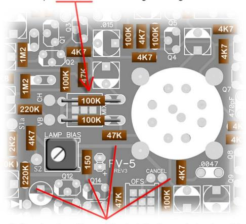
In these layout graphics, resistors look like they are laying down flat this is only so their labels can be read easy when doing your build the resistors should be installed "stand-up" style.
