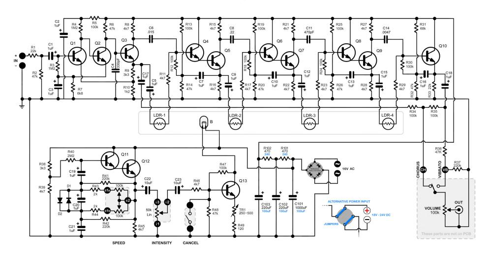
NOTE: Capacitors C101, C102, and C103 should be compact types such as Nichicon VK or VR series which are 10mm X 12mm size.
